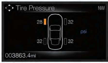
Displays tire pressure by location in psi, bar, or kPa.
