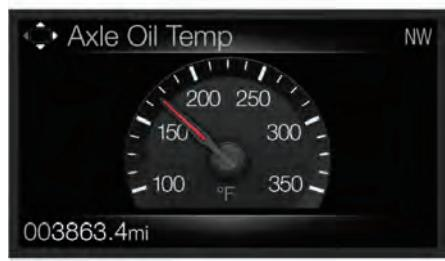
Displays the axle oil temperature.
