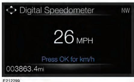
Displays vehicle speed in mph or km/h.
