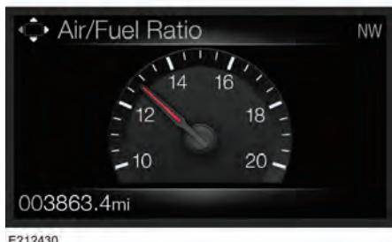
Displays the current air to fuel mixture in the engine.
