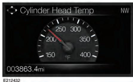
Displays the engine cylinder head temperature.
