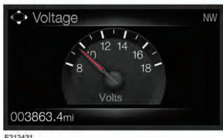
Displays the vehicle battery voltage.
