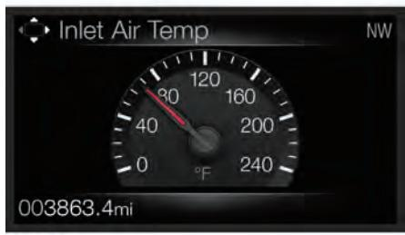
Displays the temperature of the air in the cold air inlet tube.
