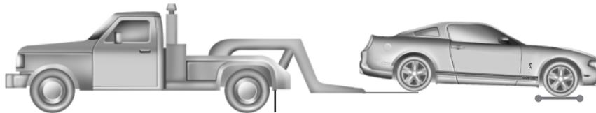
When towing the Shelby GT500, for front loading, the front tires must be 16 inches (41 centimeters) higher than the rear.
