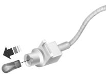
5. Carefully pull the bulb straight out of socket.
