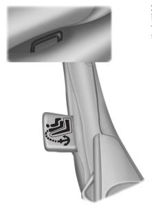
2. Access tether anchors located behind the seat back under the vinyl tag marked with the child tether anchor symbol.
