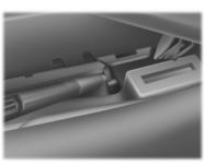
4. Press and hold the lever forward while pulling the gearshift lever out of the  $\mathbf{P}$  (Park) position and into the  $\mathbf{N}$  (Neutral) position.
