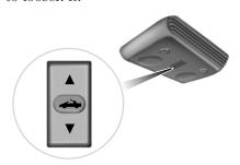
4. Press and hold the convertible top switch on the overhead console until the windows are completely down and the top is completely stored.
