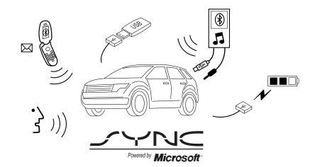
SYNC is an in-vehicle communications system that works with your Bluetooth-enabled cellular phone and portable media player. This allows you to:
