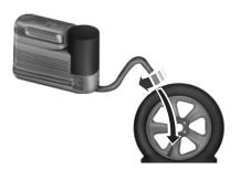
8. Inflate the tire to the pressure listed on the Tire Label located on the driver's door or the door jamb
