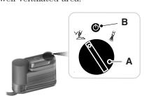
7. Push and turn dial (A) counterclockwise to the sealant position. Turn on the kit by pressing the on button (B).
