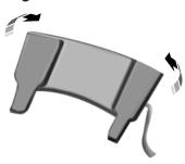
1. Position the boot right-side up and fold each side of the boot inward.
