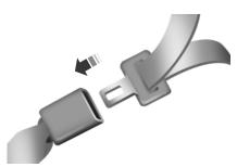
1. Insert the belt tongue into the proper buckle (the buckle closest to the direction the tongue is coming from) until you hear a snap and feel it latch. Make sure the tongue is securely fastened in the buckle.
