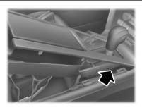
3. Lift the center console upward to access the base of the gear shifter assembly and locate the brakeshift interlock override lever.
