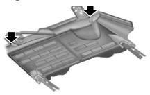
Some vehicles may be equipped with an aero-shield under the engine. Remove the front fasteners of the shield to gain access for service. This includes oil and filter changes.
