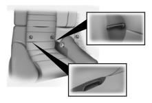
The LATCH anchors are located at the rear section of the rear seat between the cushion and seat back below the symbols as shown. Follow the child seat manufacturer's instructions to properly install a child seat with LATCH attachments.
