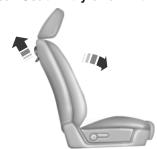
Use the seat back release to fold the back of the front seat forward for rear seat access. This release handle is located on the upper back of the front seat. The seat back locks automatically when returned to the normal position.
