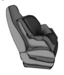
1. Position the child safety seat in a seat with a combination lap and shoulder belt.
