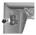
1. Inside the vehicle, pull the hood release handle located on the driver's side kick panel.
