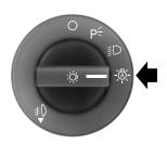
The autolamp system provides light sensitive automatic on-off control of the exterior lights normally controlled by the headlamp control.
