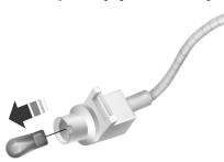
4. Carefully pull the bulb straight out of socket.
