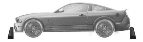
Your vehicle is designed for high speed capability and has been aerodynamically tuned to reach 200 mph (322 km/h) when properly equipped. Some of the aerodynamic tuning has been achieved with the lower front air dam, which is attached below the front splitter. The lower front air dam is removable with basic tools to suit your driving conditions, especially if they include steep driveway angles, rough roads, high curbs or harsh climates.
