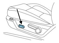
Move the switch in the direction of the arrows to raise or lower the front portion of the seat cushion.
