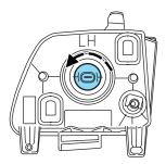
warning: Handle a halogen headlamp bulb carefully and keep out of children's reach. Grasp the bulb only by its plastic base and do not touch the glass. The oil from your hand could cause the bulb to break the next time the headlamps are operated.
