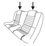
**Note:** The attachments for the convertible boot located on the back of the head restraints are not tether anchors.
