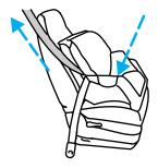
snugness of the child seat to the vehicle. Sometimes, a slight lean towards the buckle will additionally help to remove remaining slack from the belt.
