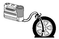
Note: When the sealing compound is first added into the tire, the air pressure gauge reading on the compressor unit may indicate a higher value; this is normal and should be no reason for concern. The pressure will drop after about 30 seconds of operation. The tire pressure has to be checked with the compressor in the OFF position to get the correct tire pressure reading.
