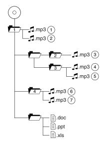
In track mode, the system will display and play the structure as if it were only one level deep (all .mp3 files will be played, regardless of being in a specific folder). In folder mode, the system will only play the .mp3 files in the current folder.
