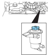
5. If the fluid is low, add fluid in small amounts, continuously checking the level until it reaches the range between the MIN and MAX lines. Be sure to put the cap back on the reservoir. Refer to *Maintenance product specifications and capacities* in this chapter for the proper fluid type.
