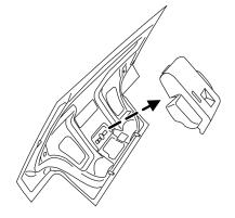
4. Carefully pull the bulb straight out of socket.
