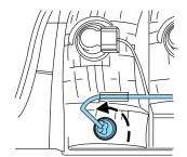
6. Pull the bulb straight from the socket.
