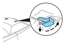
**Note:** If the top has not been lowered for some time and sticks to the windshield header, push the front of the top up slightly with your hand to loosen it.
