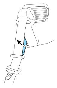
1. Insert the belt tongue into the proper buckle (the buckle closest to the direction the tongue is coming from) until you hear a snap and feel it latch. Make sure the tongue is securely fastened in the buckle.
