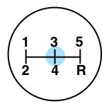
• The gearshift lever can only be moved into R (Reverse) by moving it from left of 3 (Third) and 4 (Fourth) before shifting into R (Reverse). This is a lockout feature that protects the transmission from accidentally being shifted into R (Reverse) from 5 (Overdrive).
