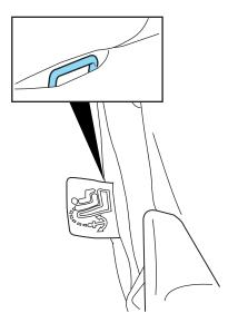
3. Clip the tether strap to the anchor as shown.
