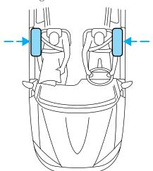
The side airbags are fitted on the outboard side of the seatbacks of the front seats. In certain lateral collisions, the airbag on the side affected by the collision will be inflated. The front passenger sensing system will turn off the passenger seat side airbag if the seat is empty. The airbag was designed to inflate between the door panel and occupant to further enhance the protection provided to occupants in side impact collisions.
