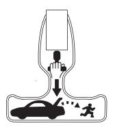
The "T" shaped handle will be located either on the luggage compartment door (lid) or inside the luggage compartment near the tail lamps.
