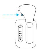
To return to normal overdrive mode, press the Transmission Control Switch again. The O/D OFF indicator light will no longer be illuminated.
