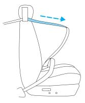
• Allow the belt to retract. As the belt retracts, you will hear a clicking sound. This indicates the safety belt is now in the automatic locking mode.
