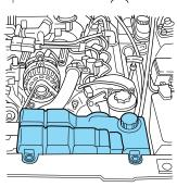
When the engine is cold, check the level of the engine coolant in the reservoir.
