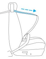
Air bags can kill or injure a child in a child seat. **NEVER** place a rear-facing child seat in front of an active air bag. If you must use a forward-facing child seat in the front seat, move the seat all the way back.
