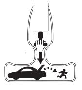
The "T" shaped handle will be located either on the luggage compartment door (lid) or inside the luggage compartment near the tail lamps.
