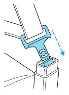
Grasp the shoulder portion and pull downward until the entire belt is extracted.
