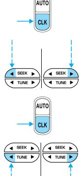
The CLK button will allow you to switch between media display mode (radio station, stereo information, etc.) and clock display mode (time). When in
