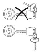
touching the **coded key** ignition key while starting the engine. These objects and devices cannot damage the **coded key** ignition key, but can cause a NO—START condition if they are too close to the key during engine start. If a problem occurs, turn ignition OFF and restart the engine with all other objects on the key ring held away from the ignition key. Check to make sure the **coded key** ignition key is an approved Ford **coded key** ignition key.
