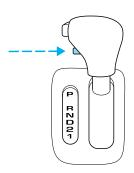
The transmission will operate in all gears except overdrive. To return to normal overdrive mode, press the Transmission Control Switch again. The O/D OFF indicator light will no longer be illuminated.
