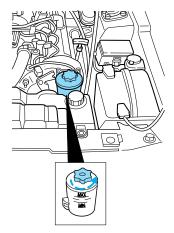
Automatic transmission fluid expands when warmed. To obtain an accurate fluid check, drive the vehicle until it is at normal operating temperature (approximately 30 km [20 miles]). If your vehicle has been operated for an extended period at high speeds, in city traffic during hot weather or pulling a trailer, the vehicle should be turned off for about 30 minutes to allow fluid to cool before checking.
