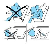
from a deploying air bag is greatest close to the trim covering the air bag module.
