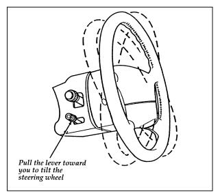
The lever to tilt the steering wheel
