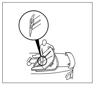
2. Push boot forward until rear attachment engages under molding.
