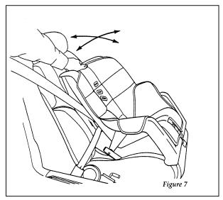
Checking that the seat is secure
