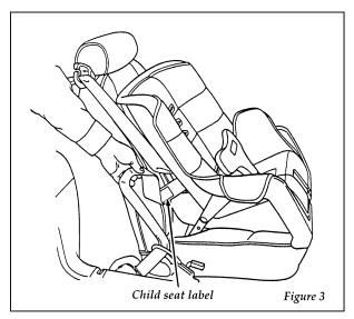
Pull the lap belt out completely to set the automatic locking mode
