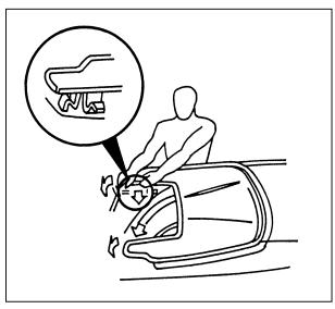
4. Tuck side attachments under molding. Repeat on other side of vehicle.
