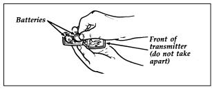
**Replacing the batteries**
