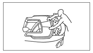
3. Push forward flap of boot until both clips engage under trim panel edge. Repeat on other side of vehicle.
