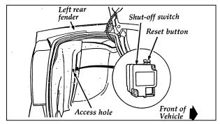
The fuel pump shut-off switch
