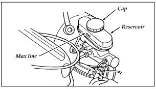
The brake fluid reservoir — 3.8L engines
