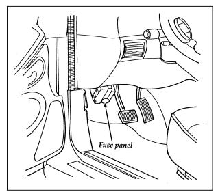
The instrument panel fuse panel location
