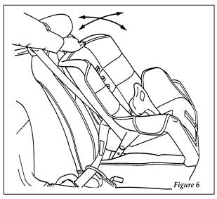
Checking that the seat is secure
