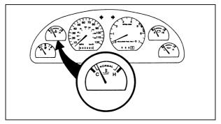
The engine coolant temperature gauge
