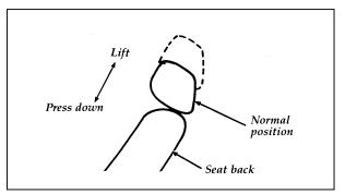
Adjusting the head restraint
