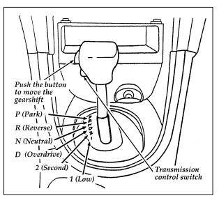
The positions of the console-mounted gearshift
