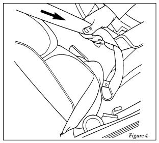
Setting the retractor to automatic locking mode
