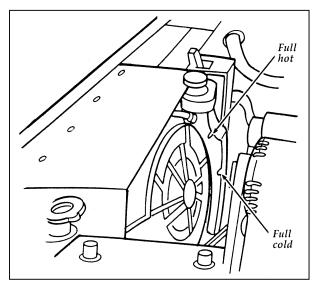
The engine coolant recovery reservoir - 3.8L
