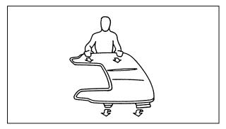
5. Push and pull front of boot to ensure tongue is engaged into groove.
