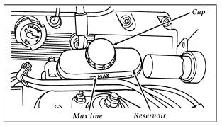
The brake fluid reservoir — 4.6L engines
