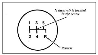
The positions of the floor-mounted gearshift
