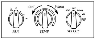
The controls for the standard heating only system
